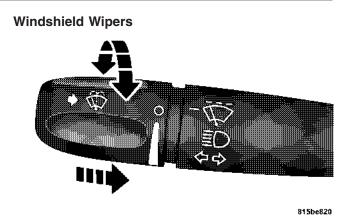
Windshield Wiper / Washer Switch The wipers and washers are operated by a switch in the multifunction control lever. Turn the end of the handle to select the desired wiper speed.
